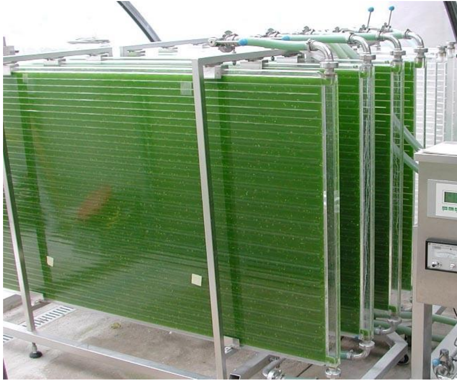
Photobioreactor for the cultivation of microalgae and other photosynthetic organisms. 2
